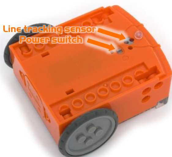
Edison's power switch and line tracking sensor
