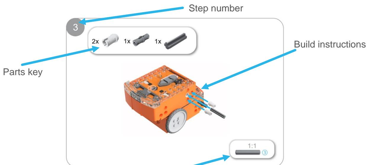
One-to-one piece measurement (when printed at 100% on A4 page). The number in the circle indicates the part's length in number of studs.
